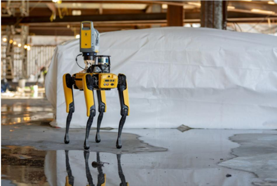
Boston Dynamics selected Velodyne Lidar's sensors to provide perception and navigation capabilities for its highly mobile robots, which are capable of tackling the toughest robotics challenges. Pictured here: Boston Dynamics' Spot mobile robot equipped with a Velodyne lidar sensor. (Photo: Boston Dynamics)
