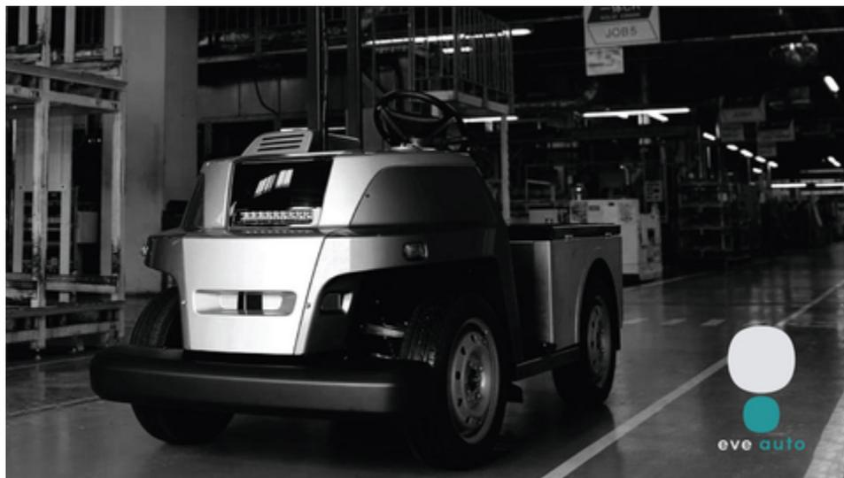
Yamaha Motor is using Velodyne's [Puck](#) lidar sensors to provide localization and navigation capabilities for their [eve auto](#) all-in-one automated conveyance service. Velodyne's lidar sensors enable the small electric vehicles to navigate factory facilities autonomously.
