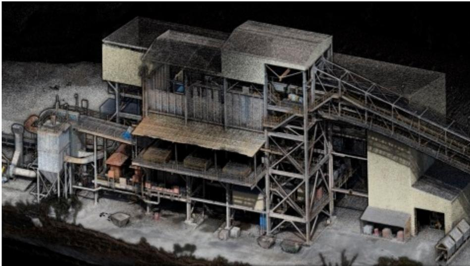
Hovermap, which can be hand-held or mounted to a drone, uses Puck LITE lidar as its primary perception and mapping sensor. Equally capable above ground or underground, indoors or out, Hovermap combines advanced collision avoidance and autonomous flight technologies to map challenging, inaccessible areas. Hovermap has a colorization feature for its 3D point clouds that brings additional context for visualization and analysis.
