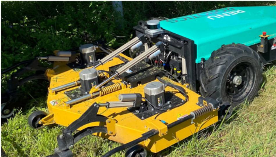
Renu Robotics' Renubot is a fully autonomous, all-electric mower equipped with Velodyne Lidar's Puck™ sensors. (Photo: Renu Robotics)
